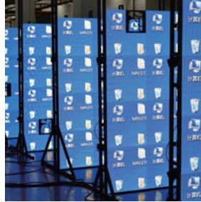
Display Aging Test
