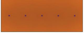
Direct sound at 1kHz obtained with 6" ceiling loudspeakers spaced by 5m, installation height 5,5m: attenuation of 3dB on the edges.
