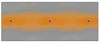
Direct sound at 1kHz on a 10m wide path with Ray-on B70TC spaced by 10m, installation height 5, 5m; attenuation -10dB at the edges.
